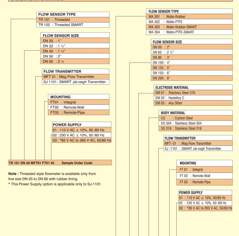
**Note:** Wafer Style flowmeter is available from line size DN 50 to DN 200. \*This Power Supply option is applicable only to SJ-1101.
