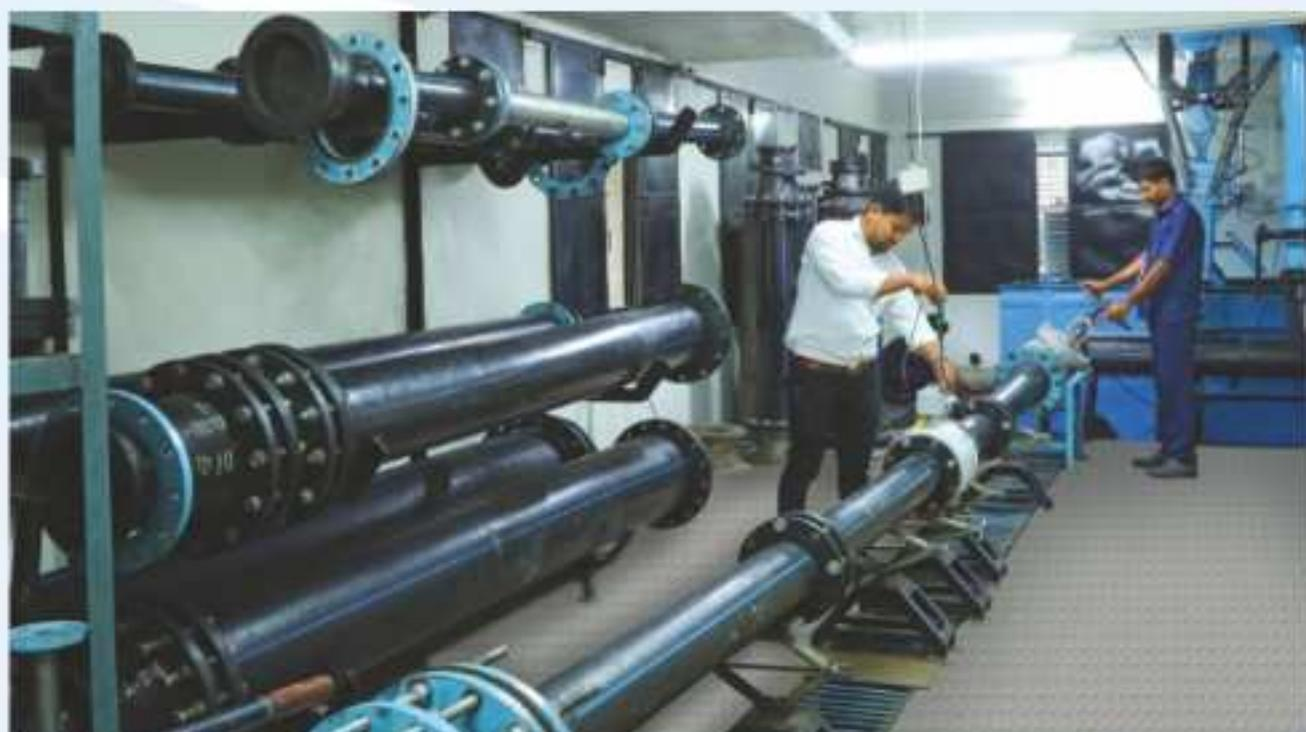
Our Liquid Calibration Lab is as per ISO 4185 Accredited by ISO/IEC 17025:2017. With setup of DN10 to DN250 with flow capacity of 0.2m<sup>3</sup>/h to 250m<sup>3</sup>/h.
