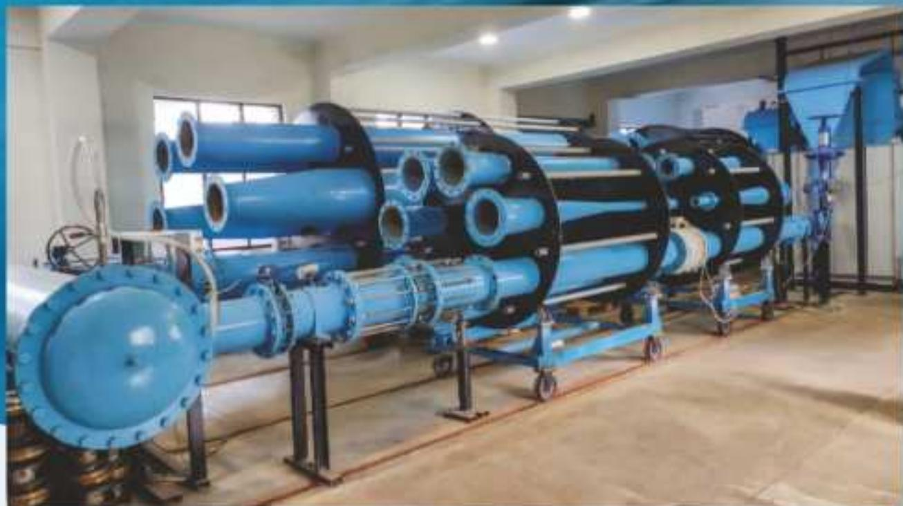
We have a flow Calibration setup up to DN600 and Max Flow Capacity up to 1000m<sup>3</sup>/hr as per ISO 4185.
